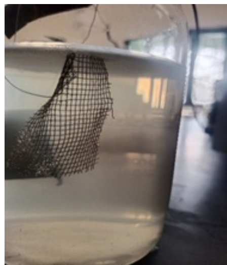
Figure 3: Cathode (Stainless Steel mesh).
